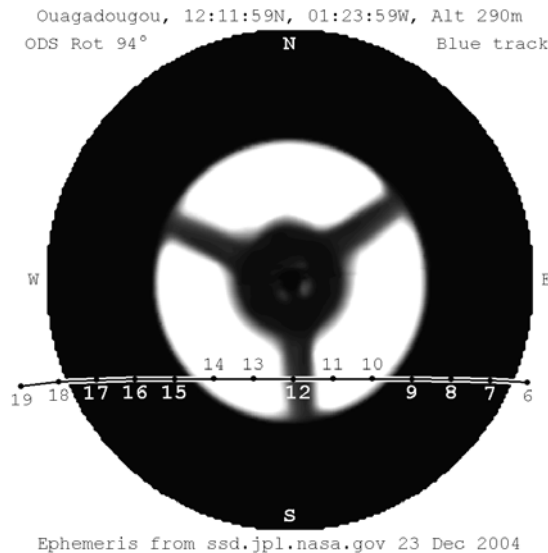
Figure V.8. Sun trajectory over the sky relative to ODS field of view on 23 December 2004 at Ouagadougou. The crossing line is the solar trajectory where the points associated with numbers along the line show the UTC time corresponding to solar positions. The background picture is the ODS field of view where white and black regions correspond to 100% and 0% transmission respectively.
