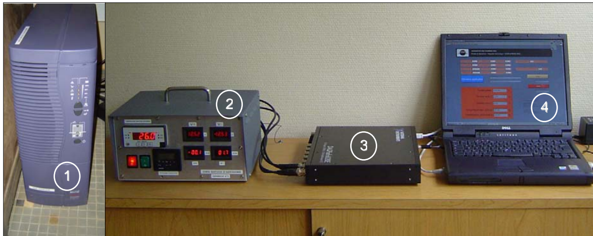
Figure V.2. Indoor acquisition chain. (1): the UPS (Uninterruptible Power Supply), (2): the GSE (Ground Supporting Equipments), (3): the DAQ (Data Acquisition Hardware), (4): Computer showing LabView interface.
