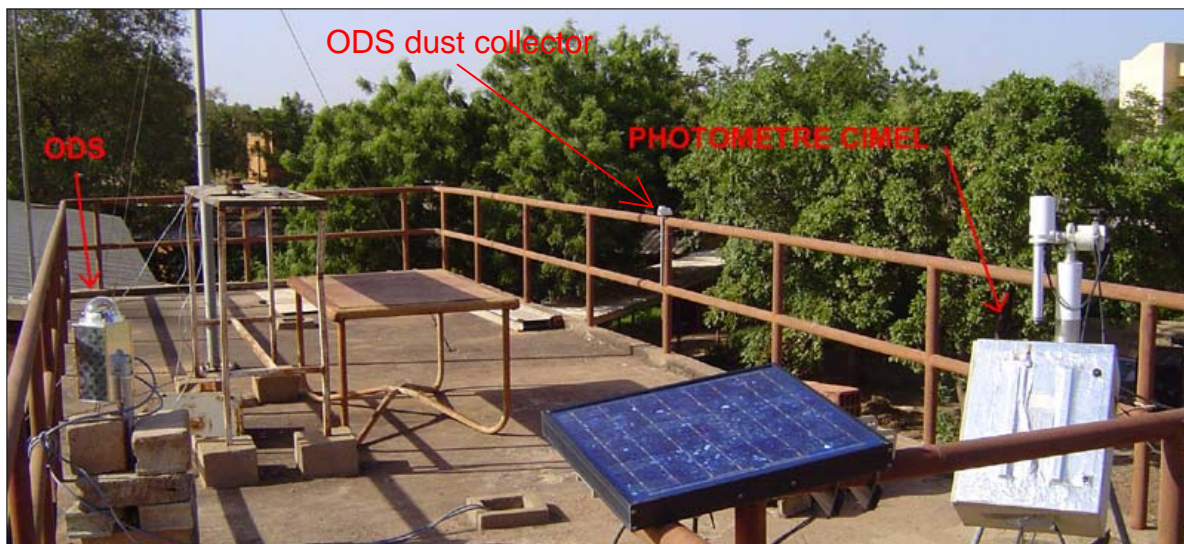
Figure V.1. ODS at Ouagadougou. The optical head is protected by the glass dome. The electronics is inside the aluminum box just underneath. The ODS is fixed firmly to a pile of bricks below. The dust collector on the right is a passive copy of ODS optics to see how much dust could deposit after a long period of exposure. The CIMEL photometer is on the forefront.
